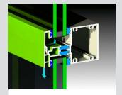
Designed to accept 24mm IGUs. Glazing pocket offers the required 12mm glass bite on İGUs. A variety of pocket closer extrusions are available should thinner glass be reauired.
